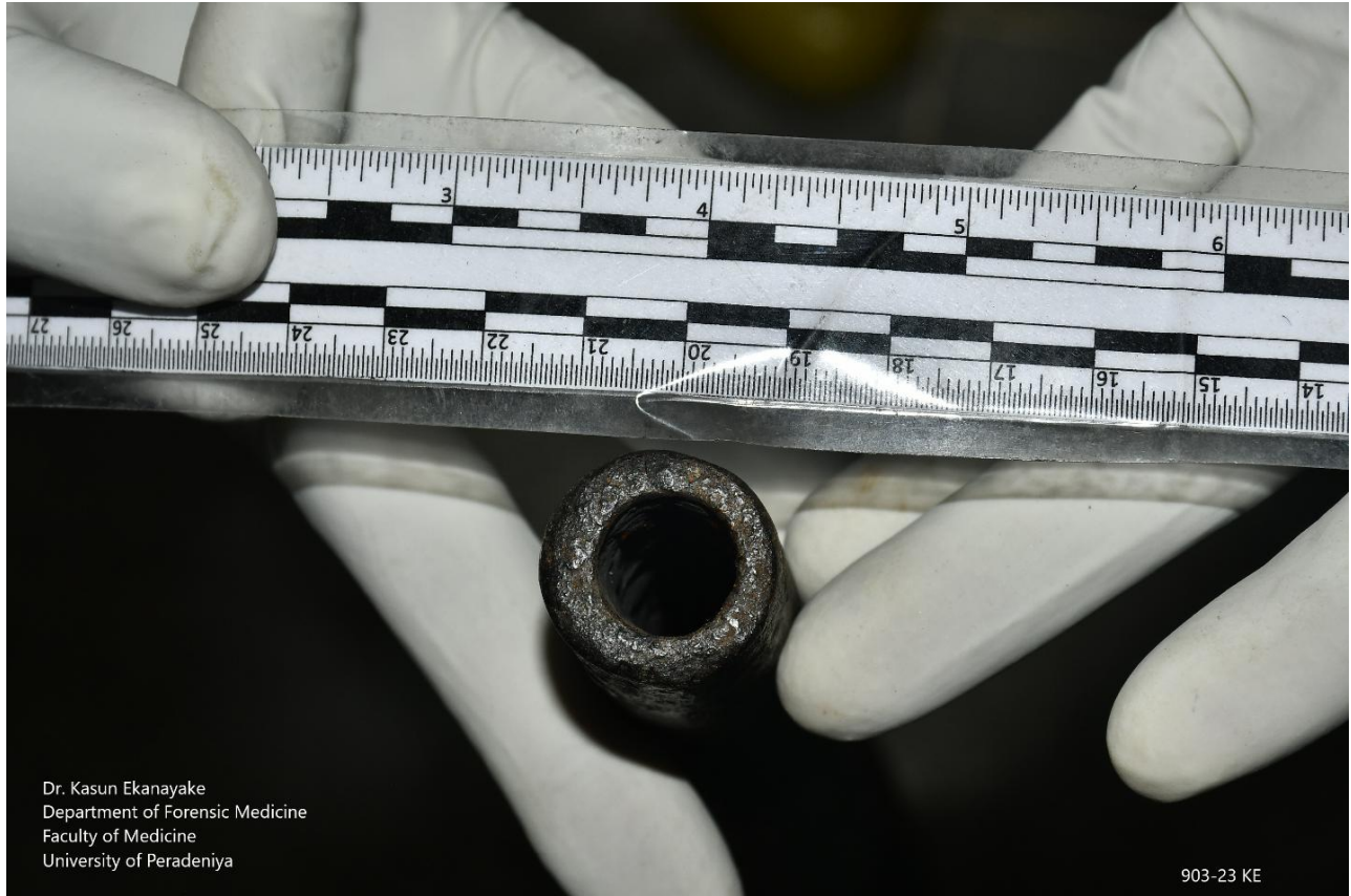
Figure 27: Smooth bore cast iron cylinder with a diameter of 15 mm.
